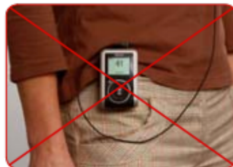
Make sure that the microphone wire does not loop under the T21.
